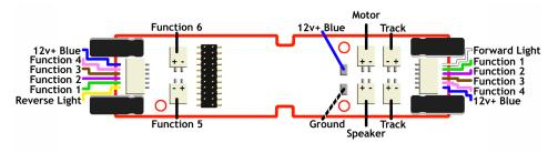
For LED's: All output functions have built-in resistors for LED's. Simply solder the negative lead from your LED to one of the function output pads (F5-F6) and then solder the positive lead to the 12v+ Common.
