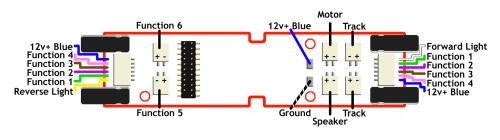
For LED's: All output functions have built-in resistors for LED's. Simply solder the negative lead from your LED to one of the function output pads (F5-F6) and then solder the positive lead to the 12v+ Common.
