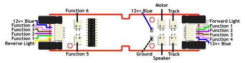
All Lighting outputs have onboard resistors for use with LED's
