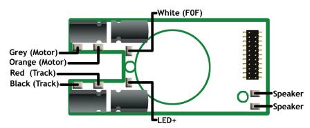
NOTE: All lighting outputs have built-in resistors for LED's
