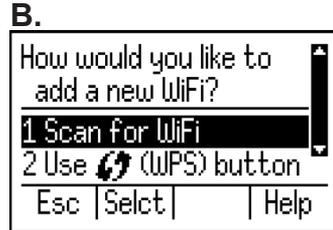
It is recommended that you use Option 1 “Scan for WiFi” to find your WiFi network - this may be a WiFi router connected to your JMRI, an LNWI, or other device (C). Once the scan is complete, the throttle will display a list of available WiFi networks. Select your desired network from the list and enter the password if necessary (D).
