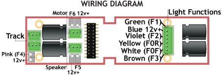
This board is a direct replacement for the Intermountain and Bowser factory light board with connectors. Simply unplug the factory light board, mount this board in its place, plug in the connectors from the locomotive, and plug in your 21-pin decoder.
