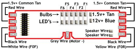
For 1.5v Bulbs: Use the F0F and F0R pads and the 1.5v+ pads. For functions F1-F6 use the bulb pads and the 1.5v+ pad.
