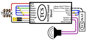
Diagram drawn for clarity - wire decoder per the written wire colors. The wires on your decoder will not be lined up the same as the diagram.
