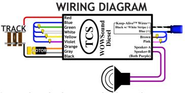
Diagram drawn for clarity - wire decoder per the written wire colors. The wires on your decoder will not be lined up the same as the diagram.
