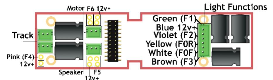
This board is a direct replacement for the Intermountain and Bowser factory light board with connectors. Simply unplug the factory light board, mount this board in its place, plug in the connectors from the locomotive, and plug in your 21-pin decoder.
