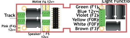
This board is a direct replacement for the Intermountain and Bowser factory light board with connectors. Simply unplug the factory light board, mount this board in its place, plug in the connectors from the locomotive, and plug in your 21-pin decoder.
