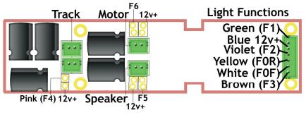
This board is a direct replacement for the Intermountain and Bowser factory light board with connectors. Simply unplug the factory light board, mount this board in its place, plug in the connectors from the locomotive, and plug in your 21-pin decoder.
