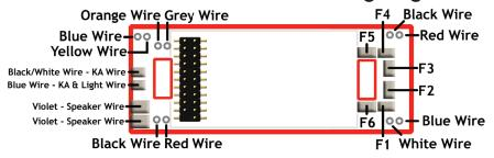
For LED's: All output functions have built-in, current limit resistors for LED's.
