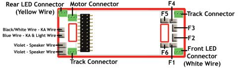
For LED's: All output functions have built-in, current limit resistors for LED's. Directly plug in the connectorized lighting leads from your engine.
