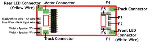
**For LED's:** All output functions have built-in, current limit resistors for LED's. Directly plug in the connectorized lighting leads from your engine.
