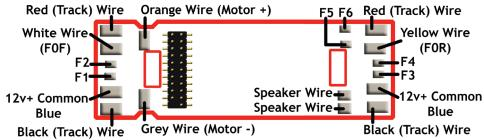
For LED's: All output functions have built-in resistors for LED's. Simply solder the negative lead from your LED to one of the function output pads (F0F-F6) and then solder the positive lead to the 12v+ Common.
