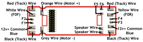
**For LED's:** All output functions have built-in resistors for LED's. Simply solder the negative lead from your LED to one of the function output pads (F0F-F6) and then solder the positive lead to the 12v+ Common.
