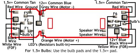
For LED's: For functions F0-F4 use the LED pads and the 12v+ pad. F5 and F6 are LED only so use their pads and the 12v+ pad. Resistors are onboard for F0-F6.
