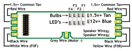
For 1.5v Bulbs: Use the F0F and F0R pads and the 1.5v+ pads. For functions F1-F4 use the bulb pads and the 1.5v+ pad.
