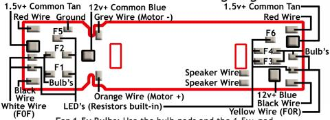
For 1.5v Bulbs: Use the bulb pads and the 1.5v+ pad.
