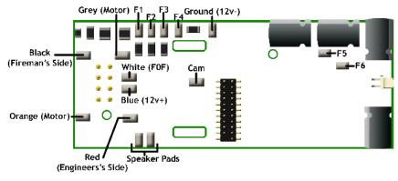
NOTE: All solder pads have in-line resistors for LED's.
