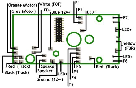
NOTE: All solder pads have in-line resistors for LED's.
