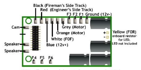
NOTE: All solder pads have in-line resistors for LED's.
