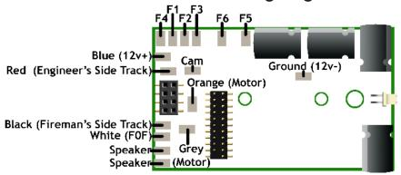
NOTE: Included on this motherboard is a rear LED light, and onboard resistors for LED's.
