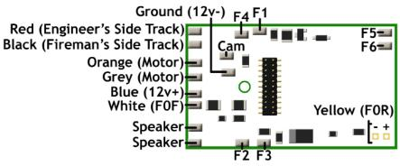
NOTE: All solder pads have in-line resistors for LED's.
