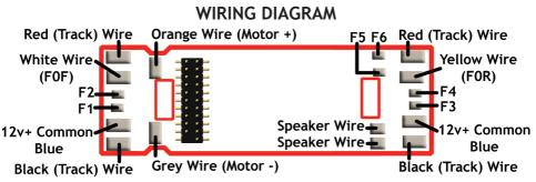
For LED's: All output functions have built-in resistors for LED's. Simply solder the negative lead from your LED to one of the function output pads (F0F-F6) and then solder the positive lead to the 12v+ Common.
