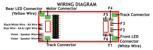
For LED's: All output functions have built-in, current limit resistors for LED's. Directly plug in the connectorized lighting leads from your engine.
