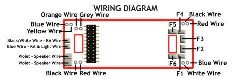
For LED's: All output functions have built-in, current limit resistors for LED's.
