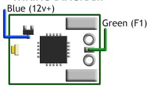
To install this decoder remove the original lighting board and slip the MT1500 into it's location.
