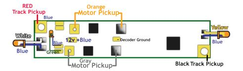
This decoder has two long motor feet on the rear end of the board.
