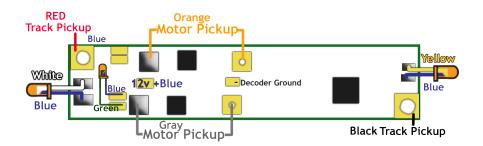
This decoder has two long motor feet on the front end of the board.
