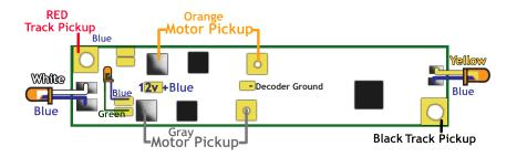
This decoder has two short motor feet on the front end of the board.
